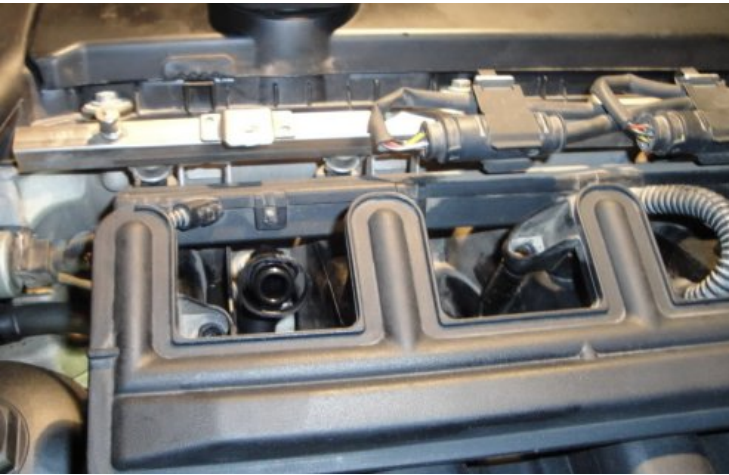
Hose routing and connections on the intake manifold.
