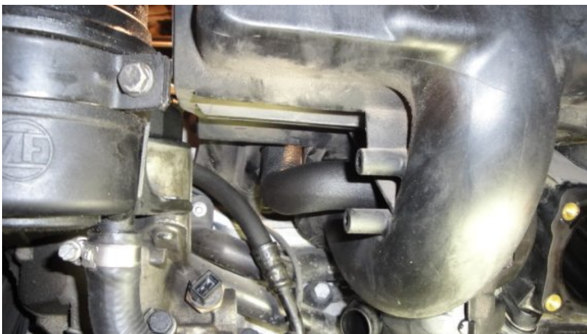
Hose routing under the intake manifold.
