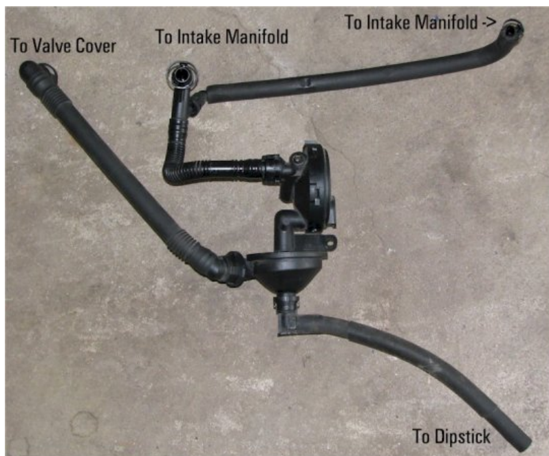
Crankcase vent system hoses.
