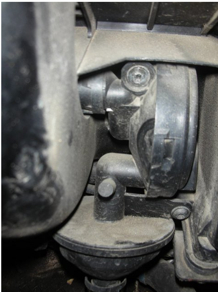
Oil Separator location on intake manifold.
